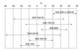
\* Can be used only when available with appropriate diesel rating. For synthetic oil use the recommendation from the oil manufacturer.
